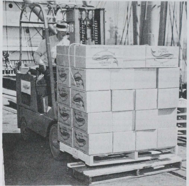
Cases of canned salmon on pallets are transported from Alaska vessel into Seattle warehouse for forklift trucks. Palletization is speeding up the transportation of canned salmon.
