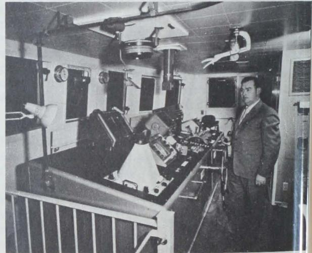
Fig. 2 - The Captain of the Acadia Albatross in the vessel's wheelhouse. In front of the Captain is an instrument console which includes radar, loran, echo-sounders, and radiotelephone. Propulsion is to be marine diesel engine and controllable pitch propeller controlled directly from the wheelhouse.
