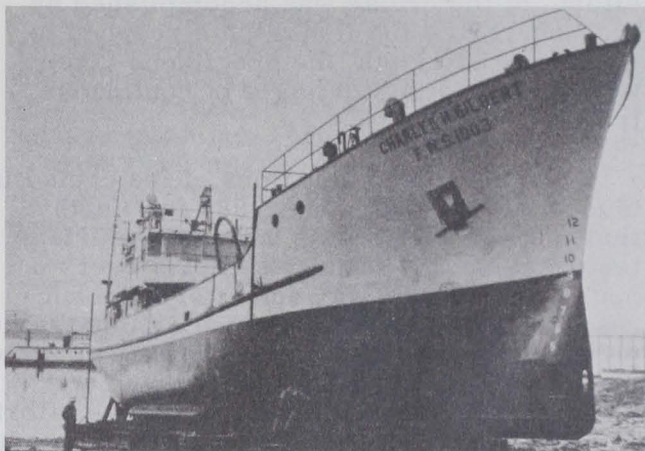
Fig. 1 - Charles H. Gilbert, research vessel of the U.S. Bureau of Commercial Fisheries. Note underwater observation chamber at the bottom of the bow end.
