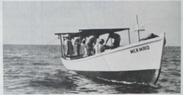
Fig. 3 - A 31-foot vessel fishing for shrimp off the Indian coast. Equipped with a 31-horsepower engine, the vessel was built to an FAO design.
