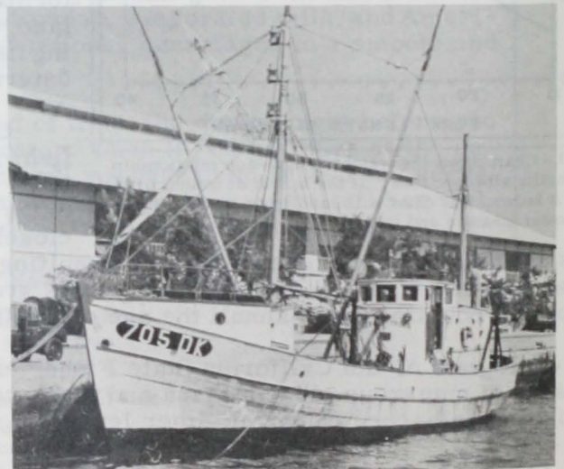
Fig. 5 - A Senegalese vessel used for trolling and trawling. The vessel was designed in 1947 by an FAO fisheries expert.
