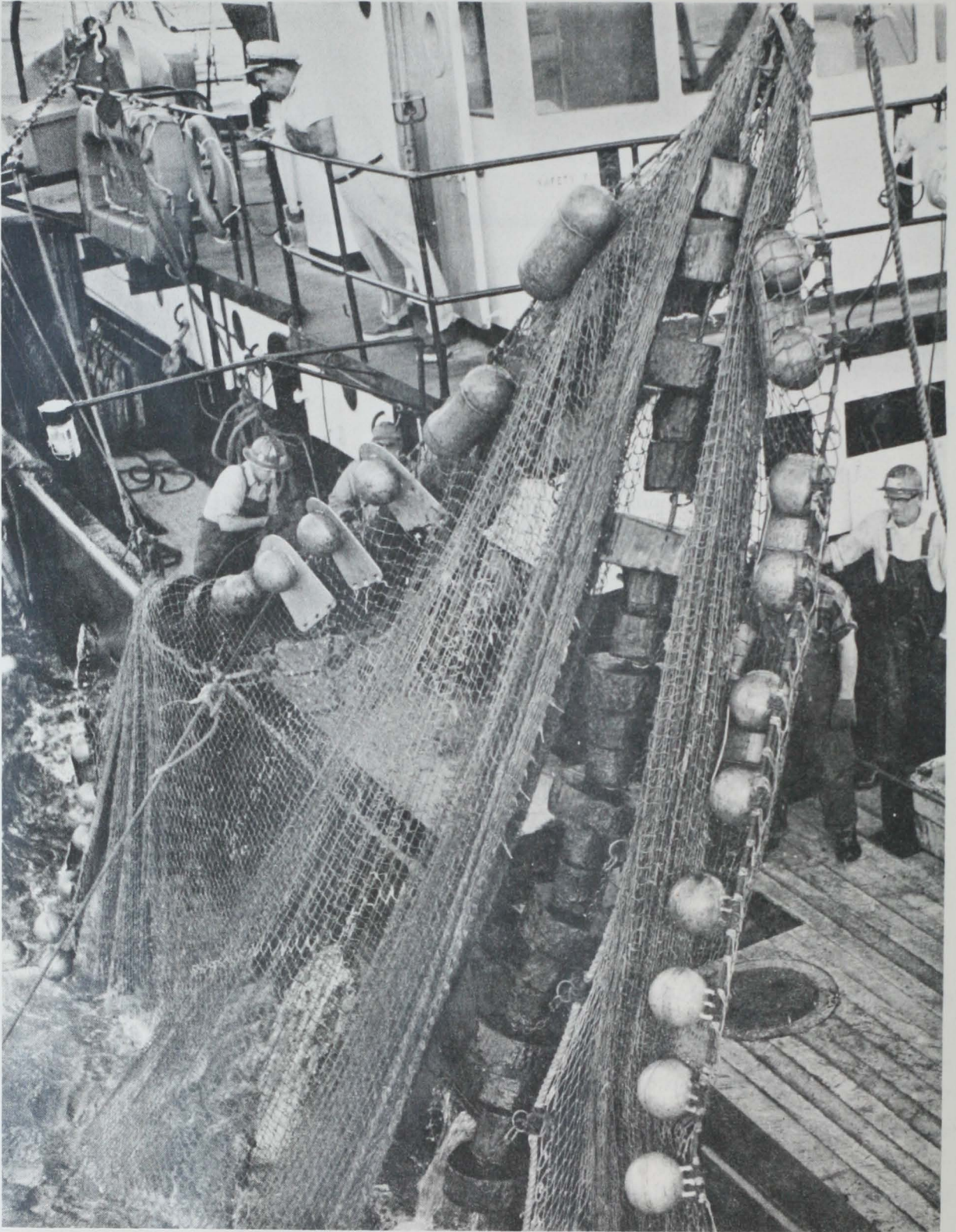
Whipping the "belly rollers" of a fish trawl aboard the "Silver Bay" during bottom fish explorations off Florida's East Coast. (Photo: J. B. Rivers)
