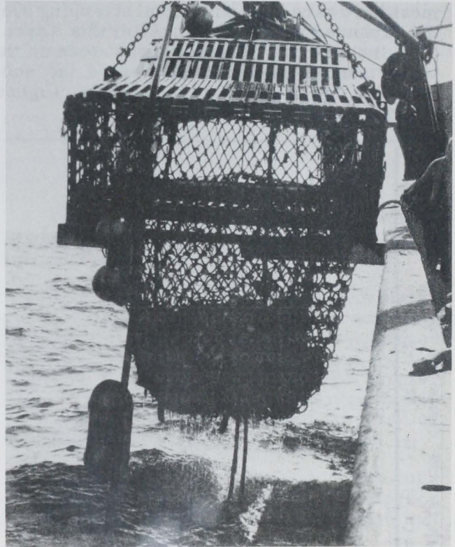
Fig. 7 - Dredge about to be taken aboard the Delaware showing catch in bag and power cable with attached floats.
