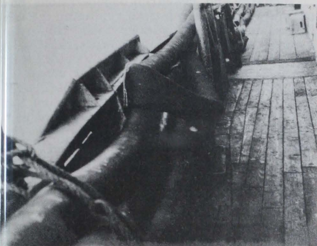
Fig. 2 - Clam jetting hose faked out aboard the Delaware.
