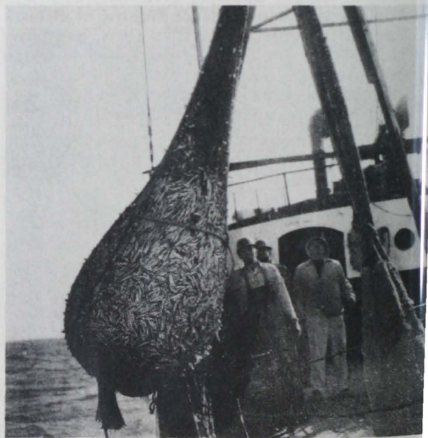
Fig. 5 - A 2500 lb. catch of round herring swinging aboard the BCF R/V Silver Bay during exploratory drags with a midwater trawl off the coast of South Carolina.
