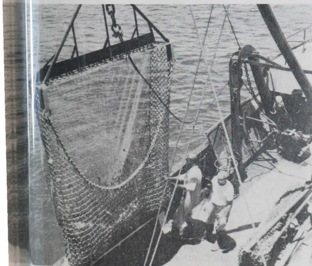
Fig. 5 - A 10' Georges Bank style scallop dredge with a catch of calico scallops swings over the railing of the BCF's research vessel "Silver Bay". (Photos 2-5: J. B. Rivers)
