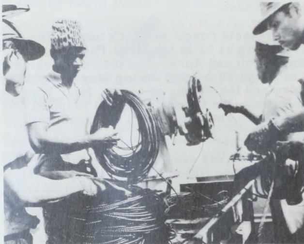
Fig. 4 - Hauling tuna longline gear aboard M/V Calamar. A crewman (2nd from right) watches coiling of mainline through mechanical hauler. Other trainees arrange a "basket" of longline gear.
