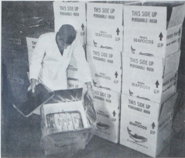
Fig. 1 - Preparing BCF insulated, leakproof, container for shipment.
