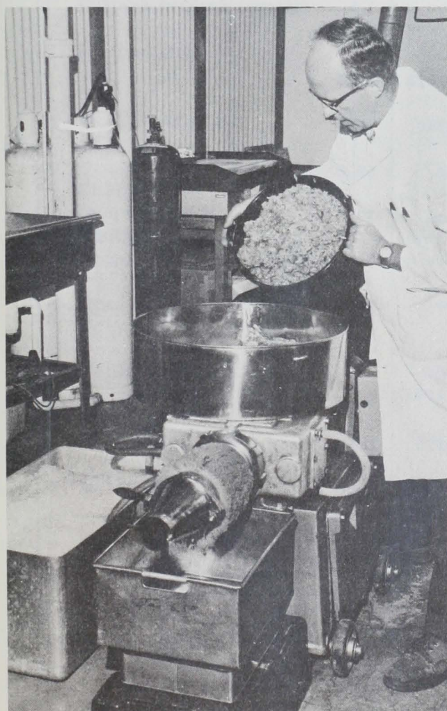
Fig. 2 - Processing machine-separated flesh through a Bibun strainer.
