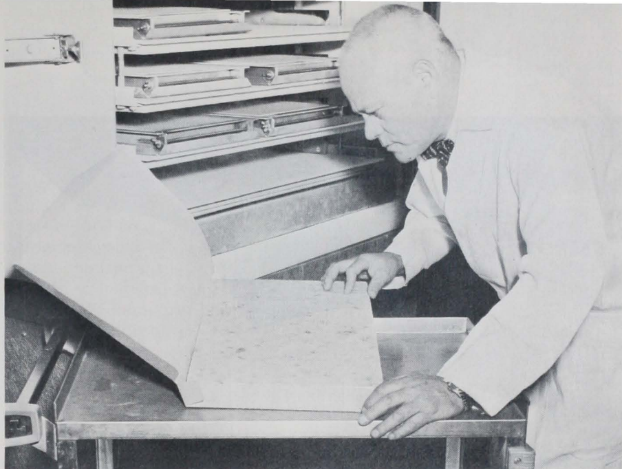
Figure 1.—A National Marine Fisheries Service scientist in Seattle examines a flavor- and texture-modified plate-frozen fish block produced from hake, one of our underutilized species. The minced flesh for this block was obtained by passing headed and gutted hake through a flesh-separator machine, at about half the cost of conventional fillets.
