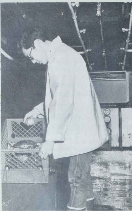
Figure 1. (above)—Live crabs in webbed basket prior to holding in fog-spray experiment. Fog-jet nozzles are shown top-center of photograph mounted between two rows of garden sprinklers.
