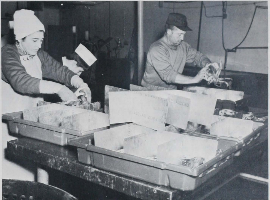
Figure 7.—Aluminum separators used to restrain crabs during tray-loading procedure.
