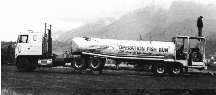
Figure 2.—Truck used to transport Pacific salmon smolts from upriver dams to a safe release site below Bonneville Dam.
