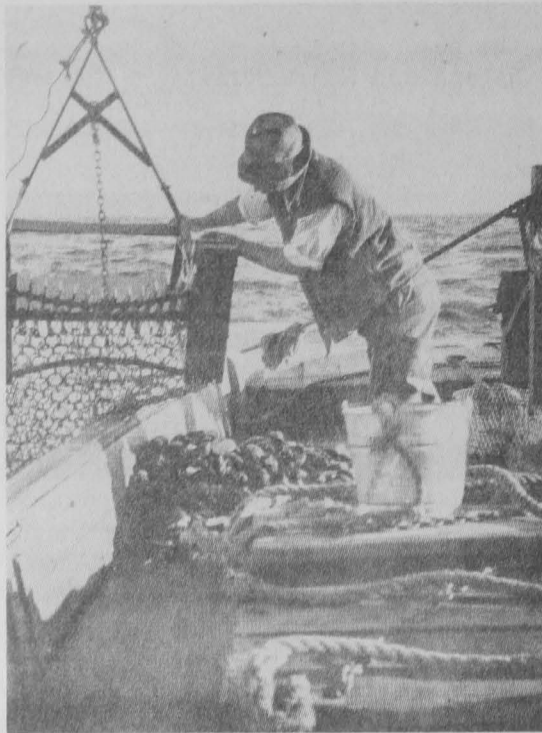
FIGURE 5B - LOWERING THE DREDGE
